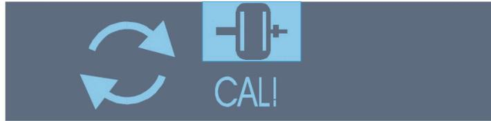
4. Spin the shaft so as to reach the rotational speed > 115 rpm. Calibration cycle starts when the shaft revolutions are brought up to the speed of 115 rpm.
