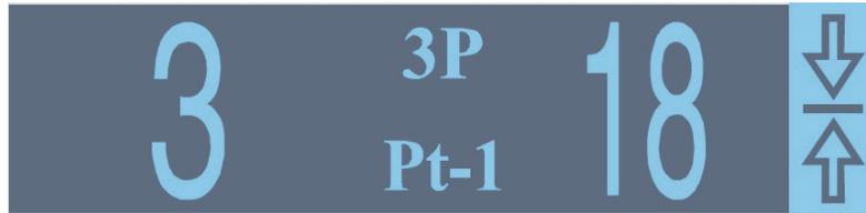
It is a position in which the correction weight of 18 g (20 g) should be stuck.
